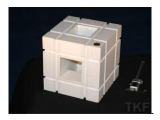
Ceramic parts are manufactured to accuracy grade per customer specification. We manufacture e. g. master angles, surface plates and straight edges as well as guideways for coordinate measuring machines. Ceramic is the material of choice due to its excellent specific stiffness, low component weight (hollow profiles) and superior thermal stability. More about: <u>Standard metrology products</u>
